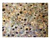
Heat Treat Response: Unibar 700-2 can be hardened by conventional methods, to Rc 50 on the bar surface, responds well to austempering (ADI). Density:
