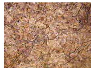
**Heat Treat Response:** Unibar 300 can be hardened by conventional methods, to Rc 50 on the bar surface.
